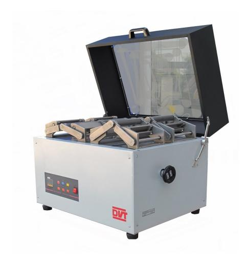
USED TO DETERMINE THE RESISTANCE OF MATERIALS (WHOLE SOLE etc.)
